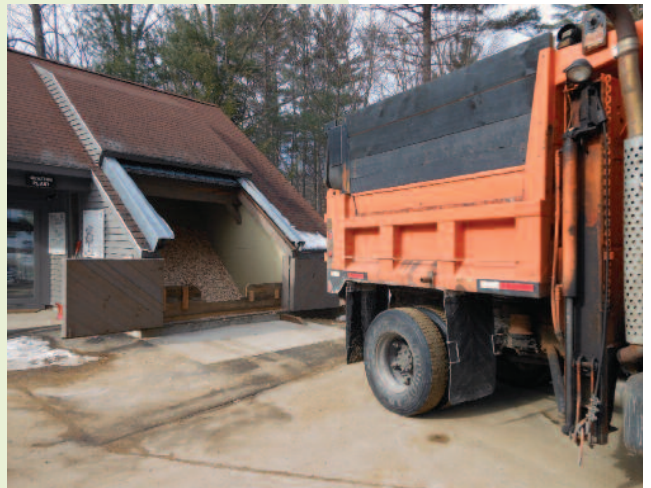
A truck gets ready to dump wood chips into the hopper at the wood-burning heating plant at the Conservation Center, the Forest Society's Concord headquarters.
